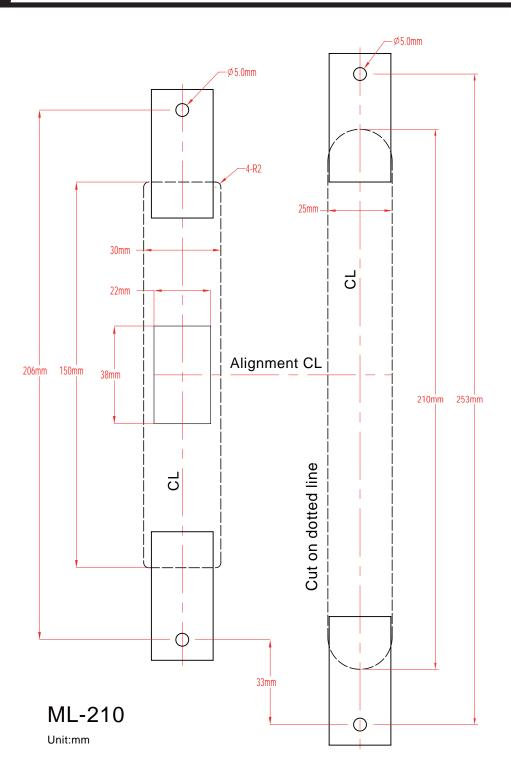
**Attention:** For "Single swing door" installation, Strike Plate and NIB can be adjusted thru the door opening and closing direction. (refer to page 1 for related NIB adjustment)
